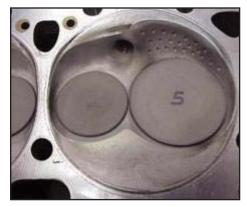
This is an alcohol-fuel small-block Chevrolet V8 combustion chamber showing uniform combustion flame patterns, aided by the dimpled places on the back wall in an area typically "washed" with fuel.
