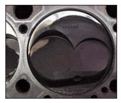
In this image, mixture motion is counterclockwise. Note separation of air and fuel as the mixture passes across the sharp edge of the intake valve pocket. Radiusing in this area would help reduce mechanical separation.
