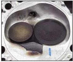
Here's another example of a fuel rich burn condition during overlap – to be avoided if possible. High exhaust gas temperatures and a reduced response to spark ignition timing changes characterize and engine in this condition.
