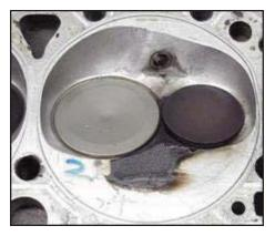
As an extreme case, this pattern reveals several unwanted conditions, including a rich condition of burn that continues into the valve overlap period, as noted by the residue between both valves. Note "clean" back wall of this chamber, a further indication of poor mixture ratios throughout the combustion space.
