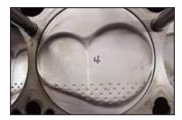
In this clockwise motion pattern, note the absence of a "clean" area in the intake valve relief. Radiusing this edge helps reduce the "edge" effect and cause of separated air and fuel in this area.
