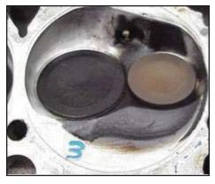
In this clockwise motion pattern, note the "clean" area on the chamber's back all, indicating air/fuel impingement and subsequent separated fuel from the air. The low-pressure area just past the spark plug encourages fuel to collect, leading to a fuel rich condition, as evidenced by the dark area. Separated fuel further "washes" past the exhaust valve, burning to a rich condition past this valve and toward the intake valve.
