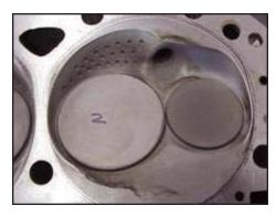
This image indicates close pistontohead proximity in the quench area (lower left-hand portion of the photo) and a slightly richer condition (compared to the remainder of the chamber's color) along the edges of this quench condition – not uncommon nor necessarily undesirable when running very tight deck clearances.
